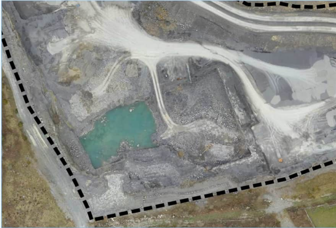
Plate 2: August 2026 - Southwest Corner (Lowest Point) of Quarry – Sump / Infiltration Area showing no water (dry)
